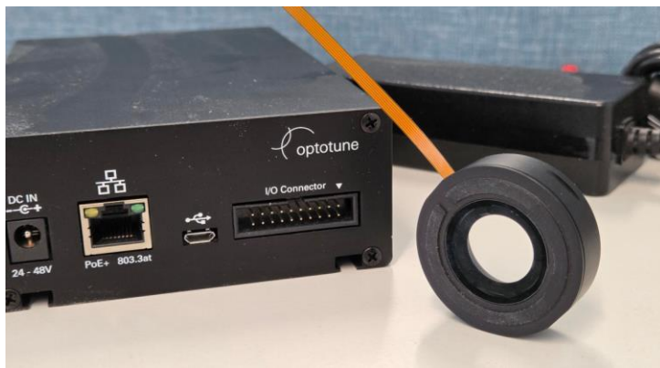
Fig 2.4: EL-16-40-GTC-VIS prototype with gravity-effect compensation.
