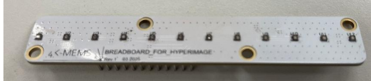
Figure 2.3.1 showing a fully mounted PCB with 12 emitter dies.
